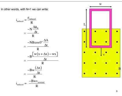
A loop of mass m, resistance R and dimension w and L falls from rest into a B-field. During the time interval before the top edge of the loop reaches the field, the loop reaches terminal velocity.
